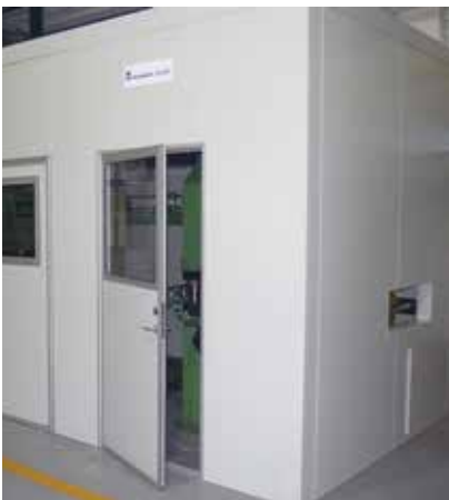
Enclosures and noise dampening for machinery at Eden Europé s.r.o, Adamov, Czech Republic.
