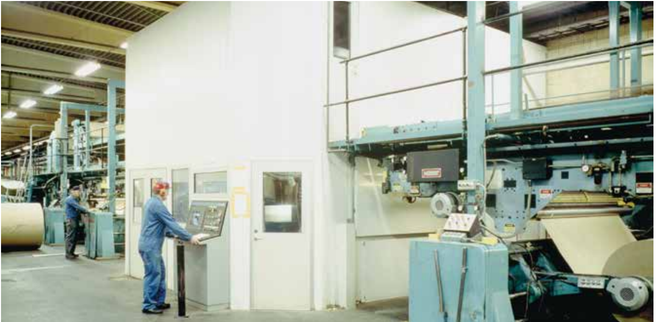
Noise-insulating enclosure, corrugated cardboard machine, SCA, Värnamo, Sweden.
